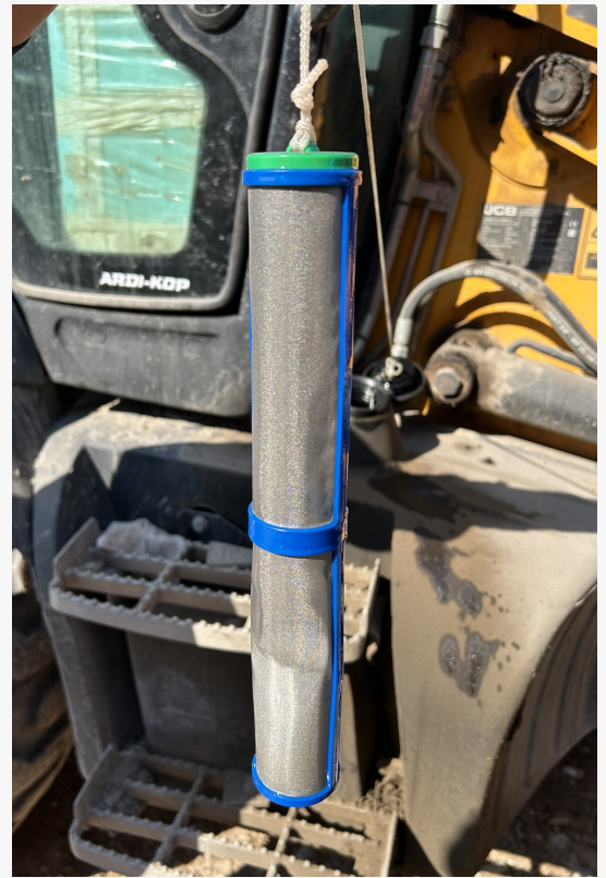
DQTube 2.0 from an excavator after one month and 50ml of water capture (50ml a month is average for diesel trucks & equipment).
