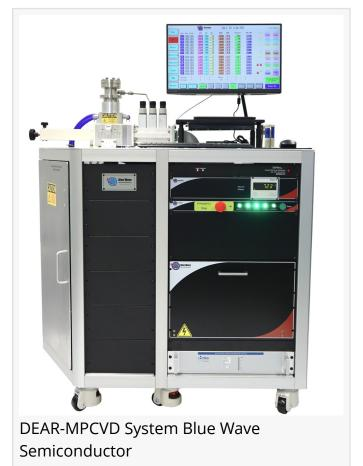
Among these, Microwave Plasma CVD (MPCVD) reactors are the most widely used for diamond growth. To enhance the properties of diamonds for electronic and quantum applications, doping is required, which can be achieved using in-situ CVD growth with the flow of dopant gas or by the ion implantation method. However, ion implantation introduces defects in the diamond lattice, making the CVD approach more suitable for device fabrication, scalability, and high-quality diamond growth.
