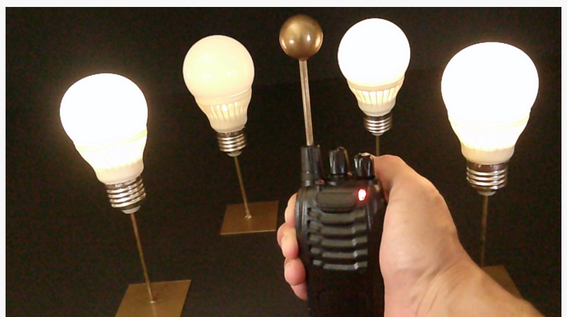
Handheld radio powering 4 bulbs
