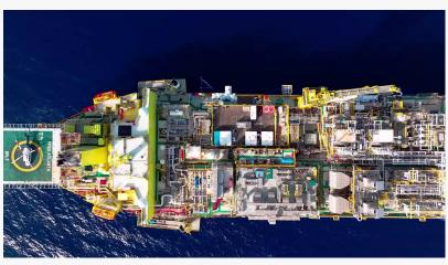
FPSO Atlanta will operate in the Atlanta field in the Santos Basin offshore Brazil. The FPSO has a production capacity of 50,000 barrels of oils per day and a maximum storage capacity of 1,200,000 barrels.
