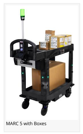
• Advanced Safety Features: Includes a 360° anti-collision system, emergency stop functions, and proximity sensors for a safer working environment.
