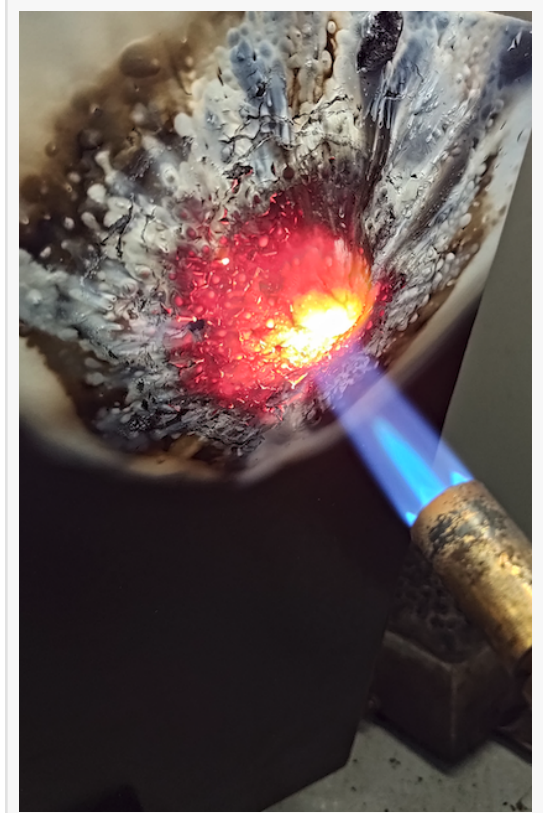
Finnester HybridRED ceramifying coatings delay ignition and reject flame spread by denying fuel that typical coatings offer to flames.
