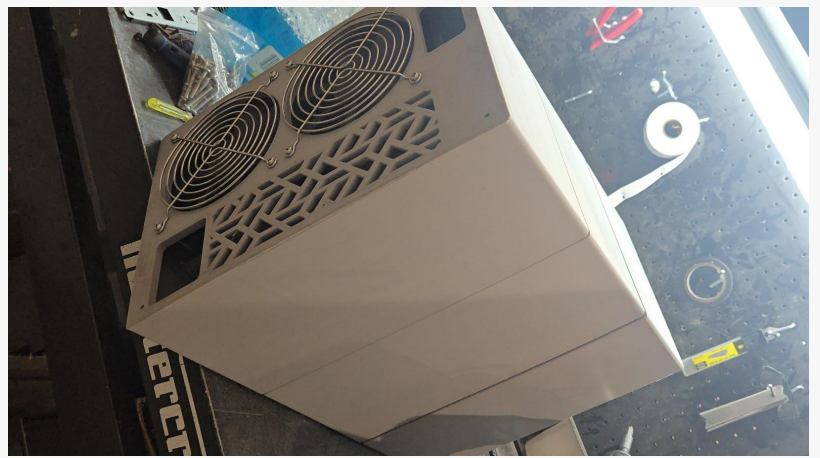
A Bitcoin Mining Heater powered by 19 Series Antminer
