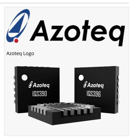
The IQS390 is a versatile haptic driver IC designed to provide highly customizable and efficient feedback through linear resonant actuator (LRA) motors. It offers two operation modes: I2C and PWM, allowing engineers to select the best mode for their applications, whether they require high-speed communication, or more control options for feedback intensity and duration. The
