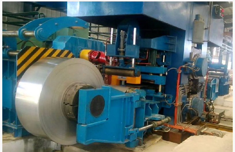
Cold Rolling Mills Machine
