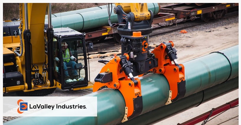
DECKHAND® material handling excavator attachment equipped with Pipe Arms.
