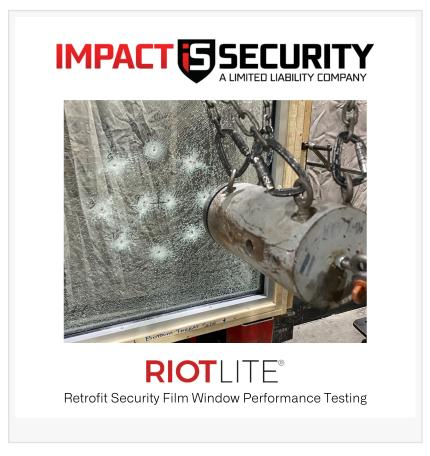
is the latest testing protocol for evaluating security window film systems against forced entry and impact scenarios. RiotLite excelled, demonstrating unmatched strength and durability in holding single pane, 1/4" (6mm) tempered glass together and delaying unauthorized entry. This achievement is critical for school administrators seeking advanced solutions to protect campuses from modern threats, including active shooter attacks on common window and door glass types.
