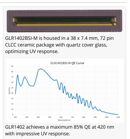
supports both sLVDS and CMOS data outputs, customer can switch different data channels with 12bit / 14bit based on demand.
