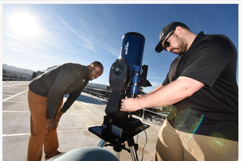
U.S. Navy Lt. Jibri Kea (left) and Kurt Heyde (right) configure tracking software for telescope to follow the Otter CubeSat to test optical communications to a ground station.
