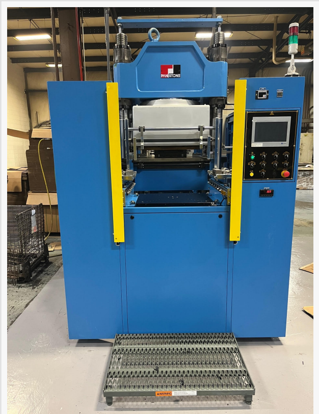
Qualiform custom rubber molding vacuum press
