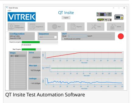
Designed to work with Vitrek's 95x, 98x and V7x series of hipot testers as well as the company's 964i high-voltage switches, QT Insite software helps automate test procedures by simplifying test design, set-up and data tracking.
