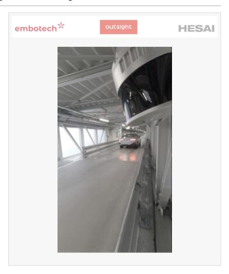
Embotech is the system provider for BMW's recently announced Auto-mated Driving In-Plant series operation and global rollout. For the AVM so-lution, Outsight plays a key role with its advanced LiDAR software platform that tracks the ego-vehicle and the surrounding obstacles within BMW's production facilities, while Hesai supplies its industry-leading LiDAR sen-sors, renowned for their accuracy and reliability, which act as the "eyes" of the AVM system.
