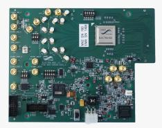
64GSPS 36GHz RF-Sampling Electra-M MX2 Evaluation Board
