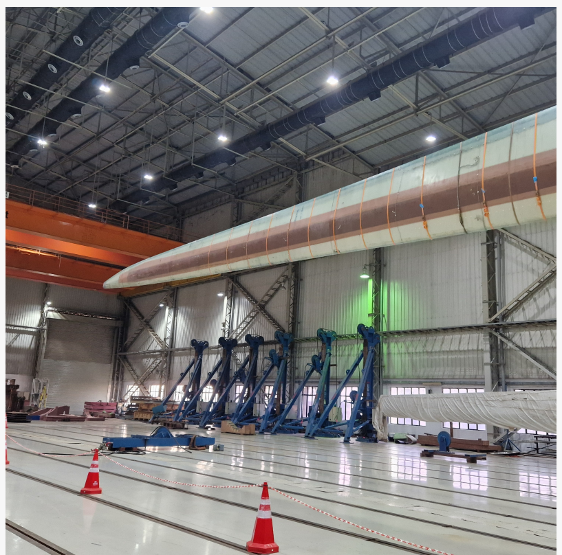
We4Ce's 2.5-3MW blade design was subjected to fatigue tests at Suzlon's test center
