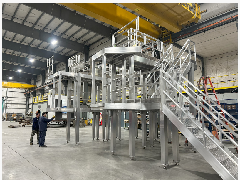
Modular Independent Spent Fuel Storage Installation (ISFSI) Platform with Swing Gate
