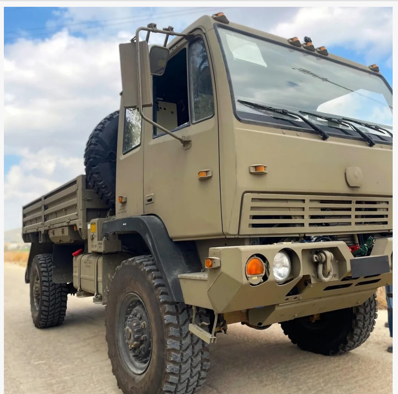
Military logistics truck converted to unmanned operation with Ottopia's kit.
