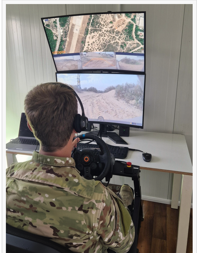
Ottopia's teleoperation station - remote vehicle control from thousands of miles away.
