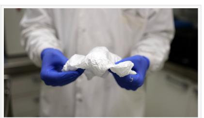
Aegis Fibretech materials provide an effective heatshielding barrier to temperatures of up to 1000 degrees Centigrade and could reduce the weight of a fire blanket to that of a couple of sheets of paper.
