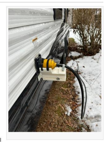
piece is comprised of a mechanism to hold the cable to relieve internal strain on the connector.
