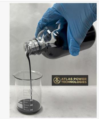
Atlas Power Technologies' NMP-free LFP slurry. This water-based formulation provides a sustainable alternative to conventional solvent-based slurries and allows for battery electrodes with customizable thicknesses.
