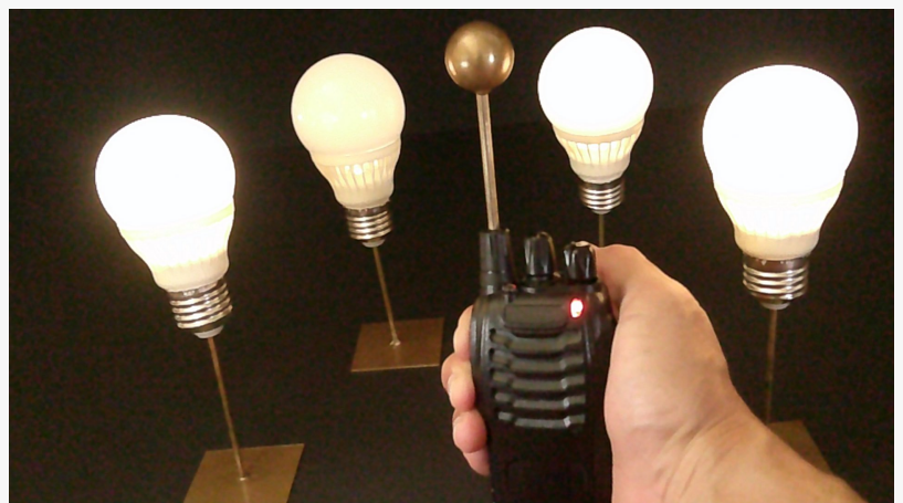
Radio powering 4 bulbs
