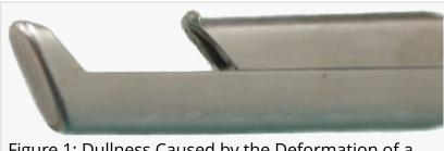
Figure 1: Dullness Caused by the Deformation of a Reusable Cutting Tip Over Time.
