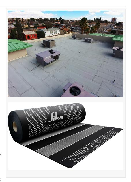
APAO polymer is compatible with SBS making the innovative combination possible. "Combining APP and SBS is the next evolution in modified bitumen membrane, says Juliana Grippa, National Manager – Bituminous Systems. "The combination of both polymers into one sheet helps form what is basically a "super membrane." The APAO top layer exhibits excellent heat resistance and durability, while the SBS bottom layer exhibits increased elongation, cold weather flexibility, and
