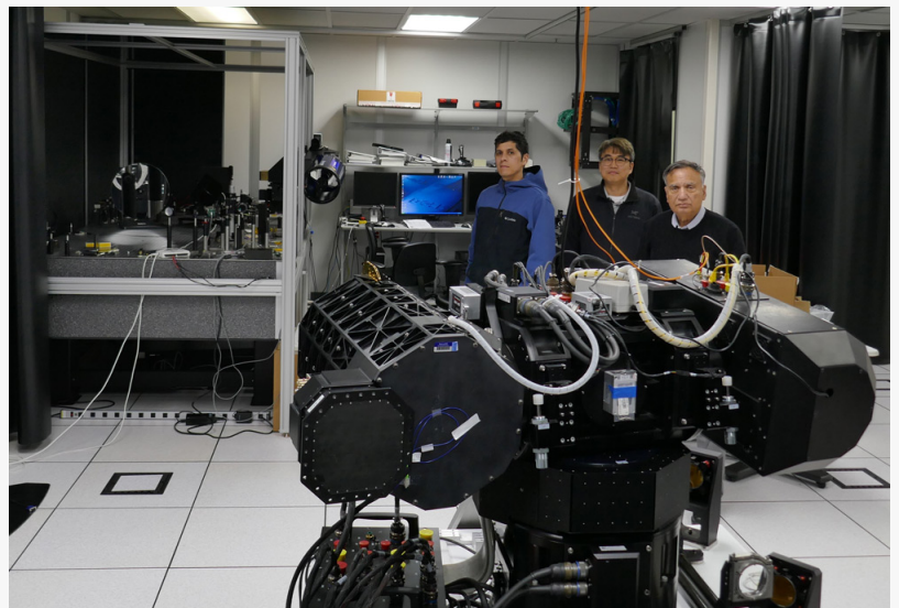
Naval Postgraduate School (NPS) researchers stand to the side of the invisible light pathway between the High Energy Laser Beam Control Research Testbed (HBCRT) and the range-in-a-box (RIAB).
