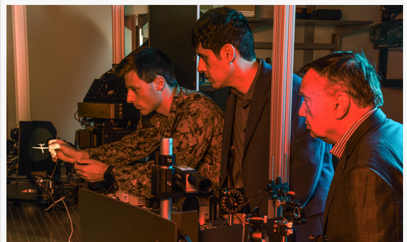
Naval Postgraduate School (NPS) faculty researchers Brij Agrawal (right) and Leonardo Herrera observe U.S. Navy Ensign Nicholas Messina positioning a Reaper drone model in an optical beam path to simulate a distant flying drone.
