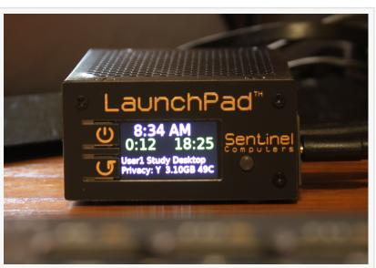
LaunchPad front panel shown with color display indicating time of day, time to screen break, remaining login time, privacy level and operating status. The front panel buttons serve many functions including power, volume, mute, login, logout and various login options.
