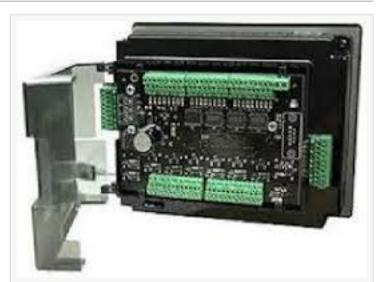
Micro and Nano Programmable Logic Controller (PLC)
