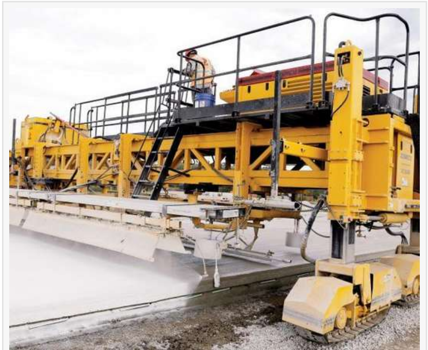
Concrete Paving Equipment
