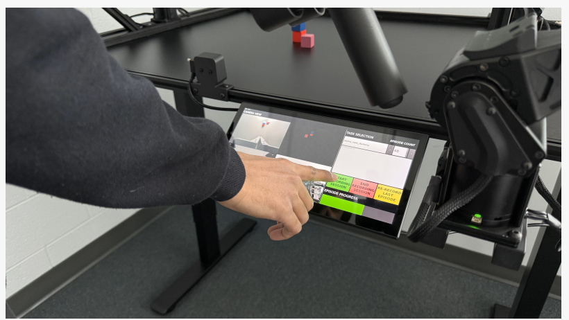
User collecting data using the touchscreen GUI interface of Trossen Stationary AI
