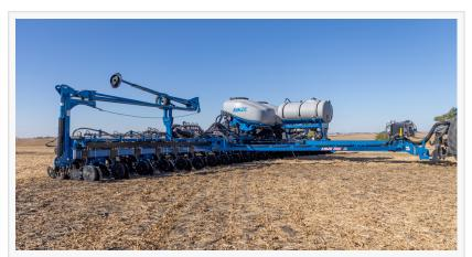
Kinze 5900 planter with dual product fertilizer system featuring row-by-row section control. Two different fertilizer products can be applied at the same time while planting and are fully controlled by Kinze Blue Vantage display.
