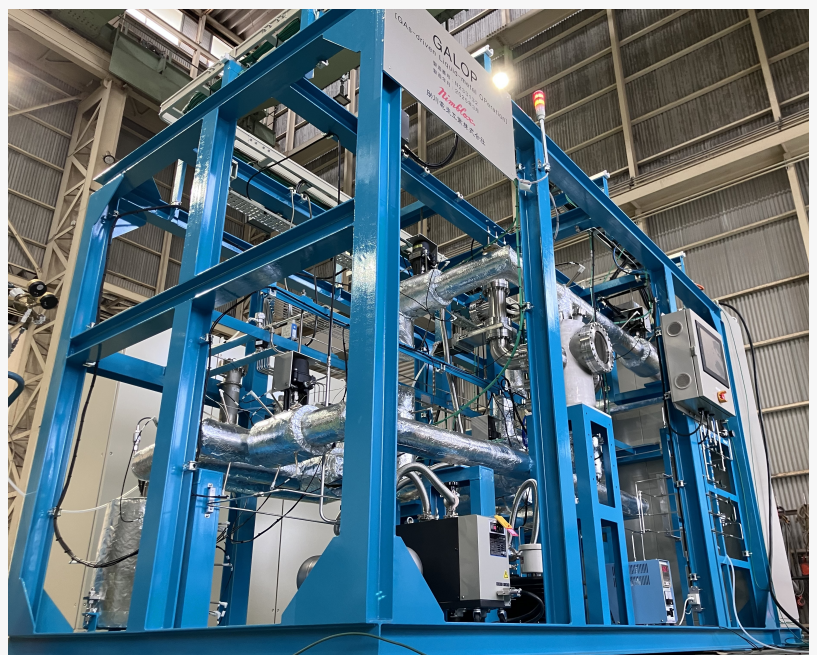
"GALOP" A Liquid Metal Blanket Testing System Essential for Commercial Fusion Reactors
