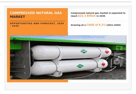
Compressed natural gas (CNG) is a type of natural gas that is compressed to a high pressure, typically between 2,900 and 3,600 psi (pounds per square inch), to make it more efficient and economical for use as a transportation fuel. CNG is a clean-burning fuel that produces lower
