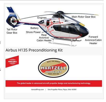
TA3391-1 – Preconditioning Kit for the Airbus H135 – 115 Voltage (USA Centric)
