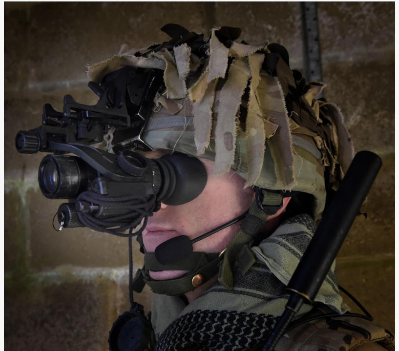
Elbit America will continue providing white phosphor image intensification tubes for use in the U.S. Army's AN/PVS-14, a monocular night vision device.
