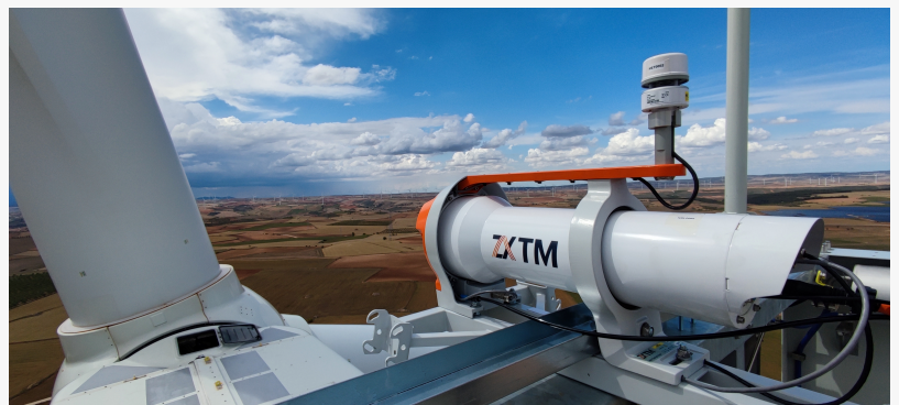
Enertis Applus+--Example of Power Curve Testing with Nacelle-Mounted LiDAR in onshore conditions"
