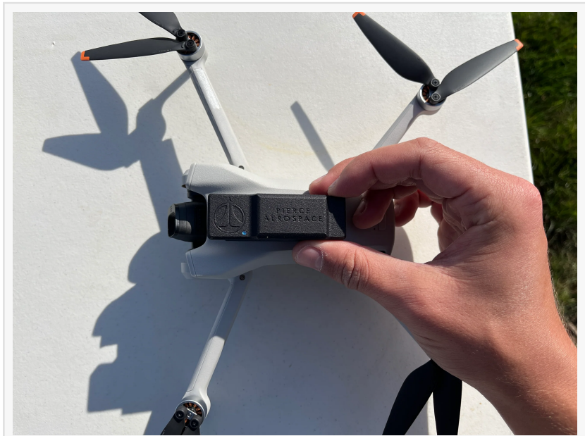
The B1 Remote ID Beacon fits nearly all drones on the market and is approved for the Blue UAS Framework.
