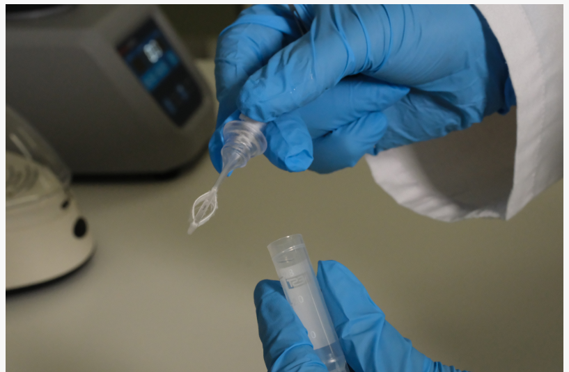
Expanded configuration of the ABEL Microsampler®, ready for laboratory processing and omics analysis
