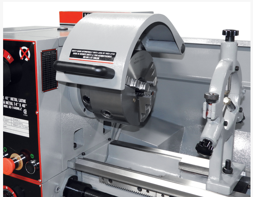
Close up of the chuck on the KC-1440ML-2
