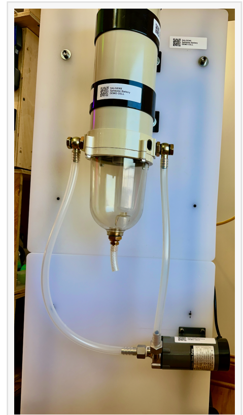
Saltwater Redox Flow Demonstration Cell
