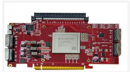
Serial Cables New Gen6 Host Interface Board with Broadcom PEX-90144-A0-1 Atlas III Switch Chip
