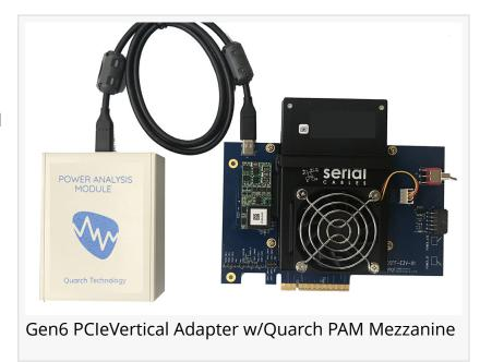
current, voltage and sidebands while the Quarch PMM is capable of manipulating the power delivery to simulate different electrical anomalies such as ramping falling or brown-out conditions
