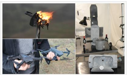
A Group 1 quadcopter burns after being engaged by Aurelius Systems' laser weapon system (LWS) during tests at the Naval Postgraduate School's (NPS) latest Joint Interagency Field Experimentation (JIFX) held Feb. 3-7, 2025.
