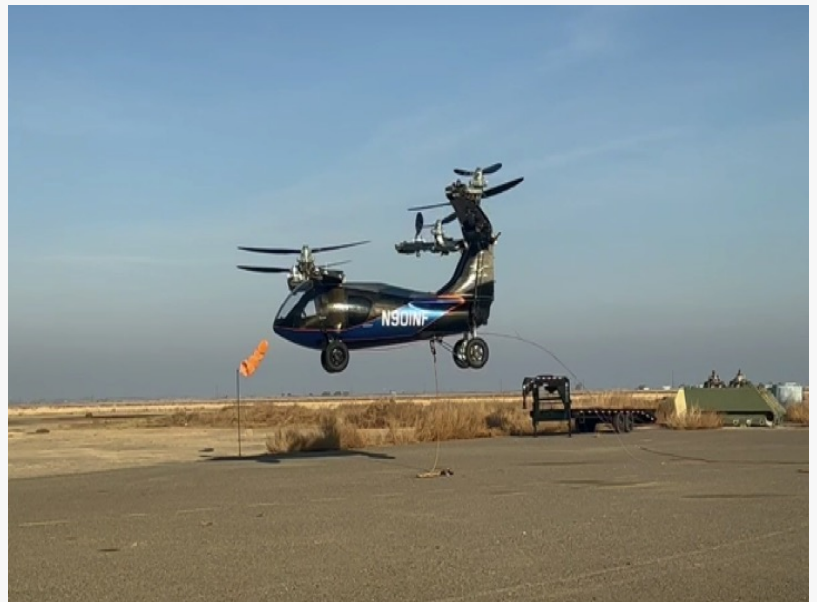
ASKA A5 tethered test flight
