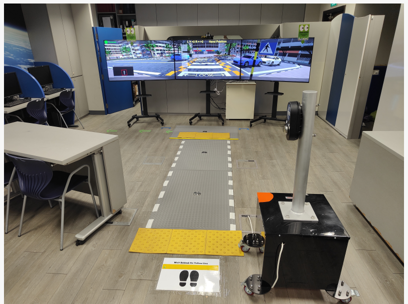
The Realistic Setup of AR-Based Road Safety Training, with Green-Man Timers, Motion-Detection Settings and Interactive Prompts
