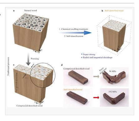
The team, led by Dafang Huang and Jie Li, used a combination of partial delignification and a LiCl/DMAc swelling process to release and reorganize wood fibers. This method allows the fibers to move inward and fill the cell lumen, followed by air-drying to achieve self-densification. Unlike traditional compressed wood, which relies on unidirectional compression, this self-densified wood exhibits uniform shrinkage in the transverse area, maintaining its longitudinal dimension.
