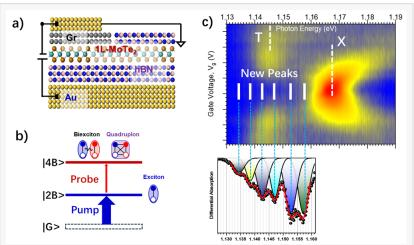
a), Device structure: a monolayer of MoTe2 is sandwiched between two thin boron nitride layers. A thin graphene layer is used for contacting MoTe2 from the top. Gate voltage is applied below the bottom boron nitride layer. b), Schematic energy scheme show
