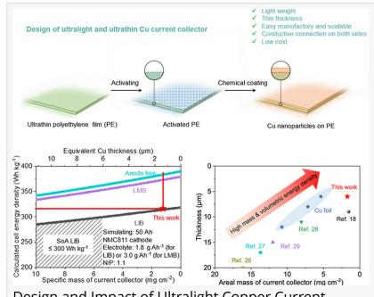
Design and Impact of Ultralight Copper Current Collectors. A schematic of the fabrication process for ultralight and ultrathin copper current collectors using a polyethylene (PE) scaffold and electroless plating.
