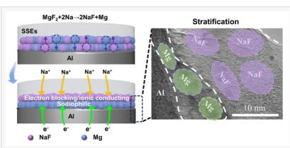
Stratified Interphase Design for Stable Sodium Batteries. This illustration demonstrates the stratified interphase in zero-sodium-excess batteries, featuring a sodiophilic magnesium (Mg) bottom layer and a sodiophobic sodium fluoride (NaF) top layer.
