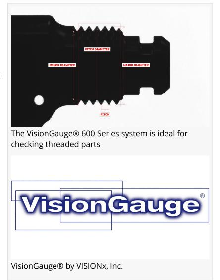
The 600 Series VisionGauge® system has the entire set of powerful VisionGauge® measurement tools. It can measure:
